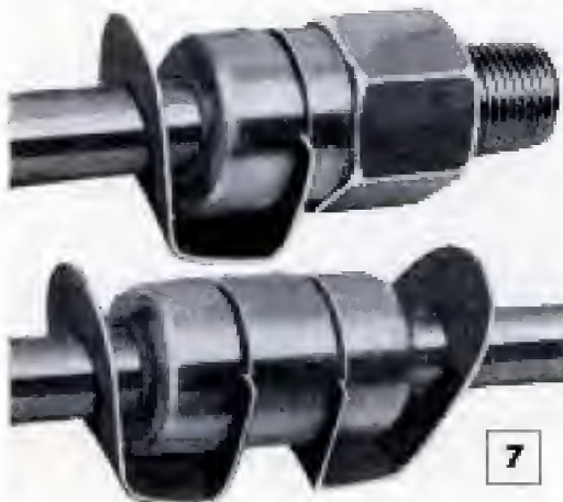
7. SPRING-CLIP CONNECTOR for tubing connections which must be liquid or gas tight, consists of a connector, or coupling and a special spring clip which is depressed as tubing is inserted. No wrenches required
